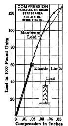
Fig. 5a.—Stress strain diagram for compression test.
